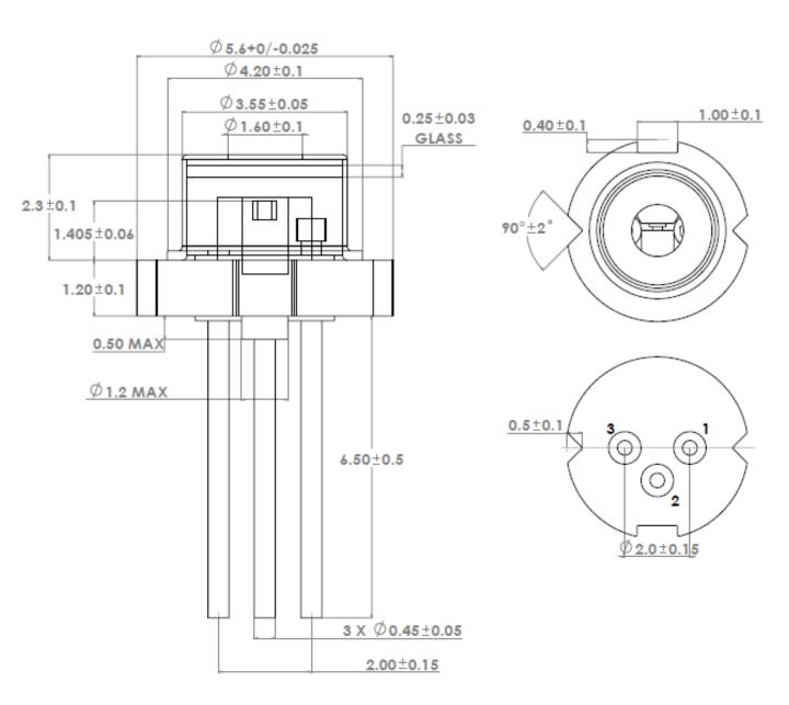
Note: Tolerance is  $\pm 0.05$ mm for items without tolerance marking
