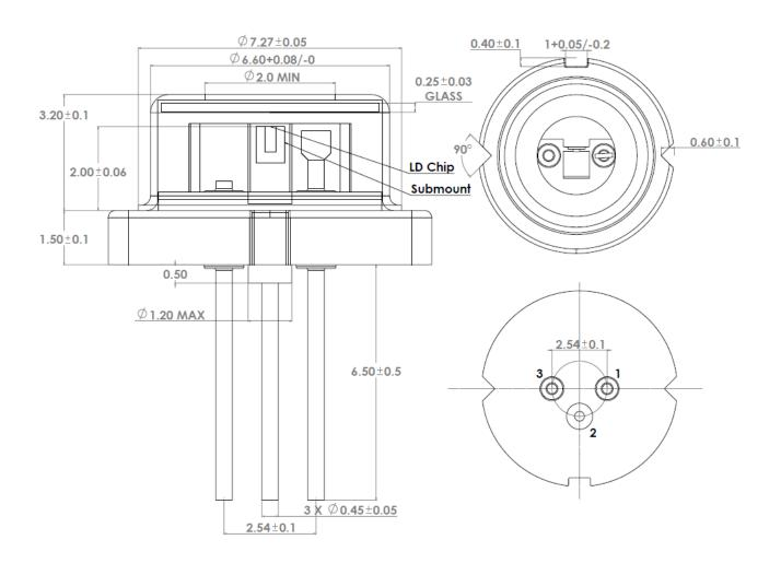
Note : Tolerance is  $\pm 0.05 \text{mm}$  for items without tolerance marking
